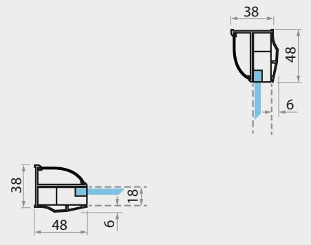
INSTALLAZIONE BOX IN RELAZIONE AL PAVIMENTO / BOX INSTALLATION IN RELATION TO THE FLOOR
