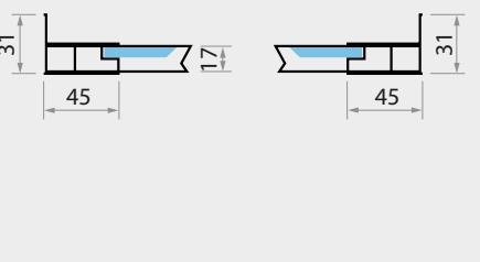
INSTALLAZIONE BOX IN RELAZIONE AL PAVIMENTO / BOX INSTALLATION IN RELATION TO THE FLOOR
