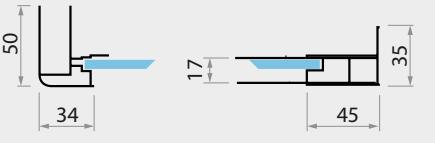
INSTALLAZIONE BOX IN RELAZIONE AL PAVIMENTO / BOX INSTALLATION IN RELATION TO THE FLOOR
