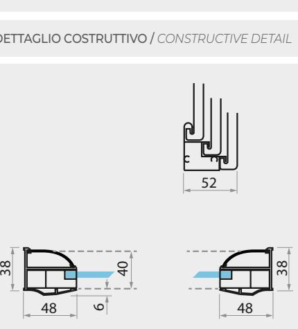
INSTALLAZIONE BOX IN RELAZIONE AL PAVIMENTO / BOX INSTALLATION IN RELATION TO THE FLOOR
