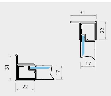
INSTALLAZIONE BOX IN RELAZIONE AL PAVIMENTO / BOX INSTALLATION IN RELATION TO THE FLOOR
