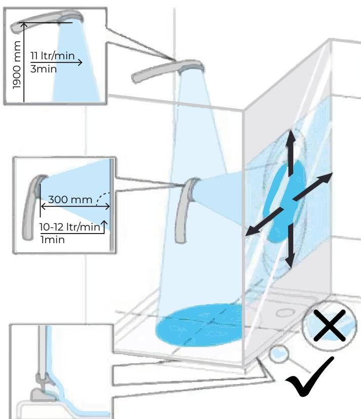
During the test, shower enclosures shall offer protection against splashing water.
